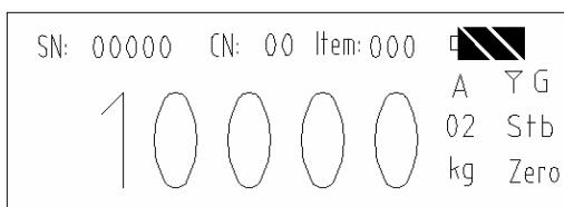
The S2 indicator uses a set of annunciators to provide additional information about the value being displayed.
