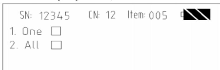
User can select deleting the weighing data one by one or deleting all the data.
